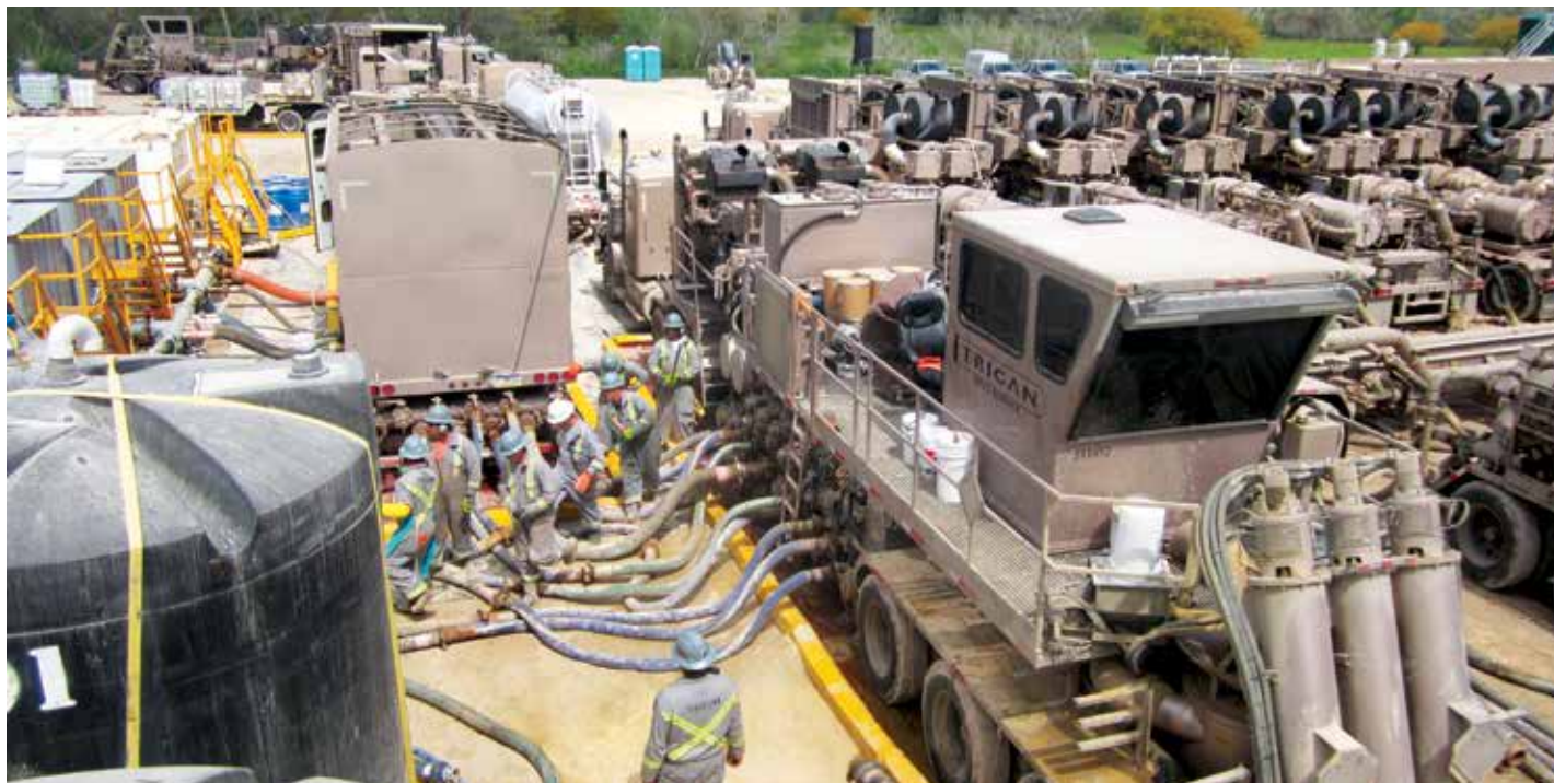
Frac blender and pumps after rig up.
