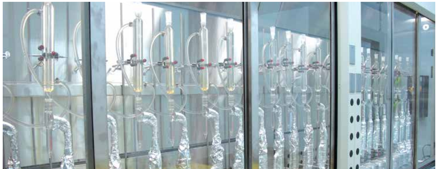
Equipment used to extract and measure the amount of water and oil stored in rock samples.
